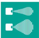
Elliptical detection area of  $\pm 17^\circ$  and  $\pm 5^\circ$
