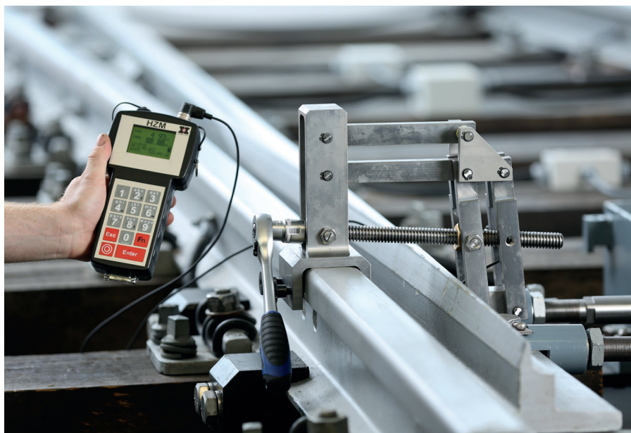
Trailing tool with force-measuring device HZM at work
